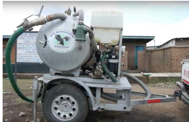
Mechanical De-sludging Units
