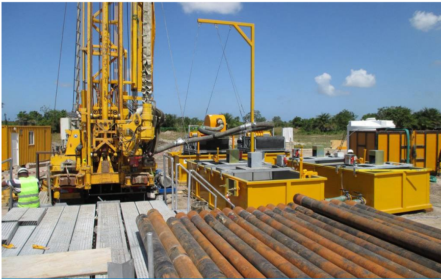
Reverse Circulation Drilling to 600m in 7 Exploration Boreholes
