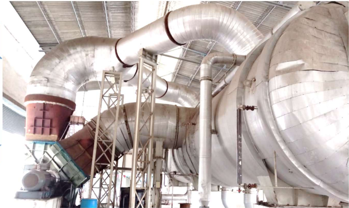
Patented Polymeric Film MVRE for 12 MLD ETP, Veerapandi, India
