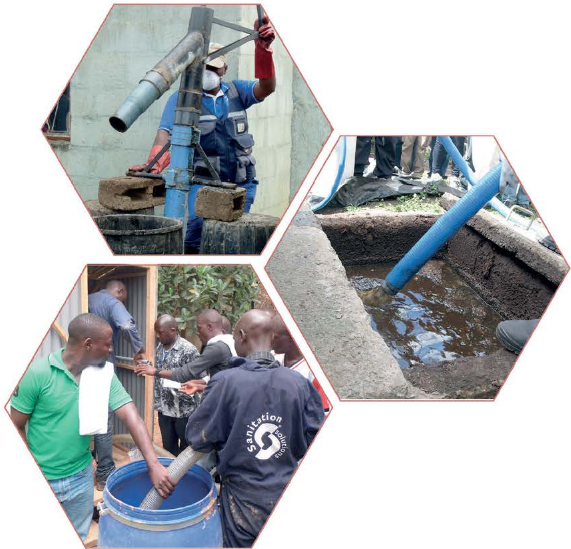
▲ Figure 11 : Use of the Gulper for FS extraction
